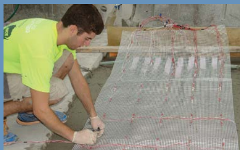
Students embed electrodes linked to a data acquisition system into “smart” concrete.
