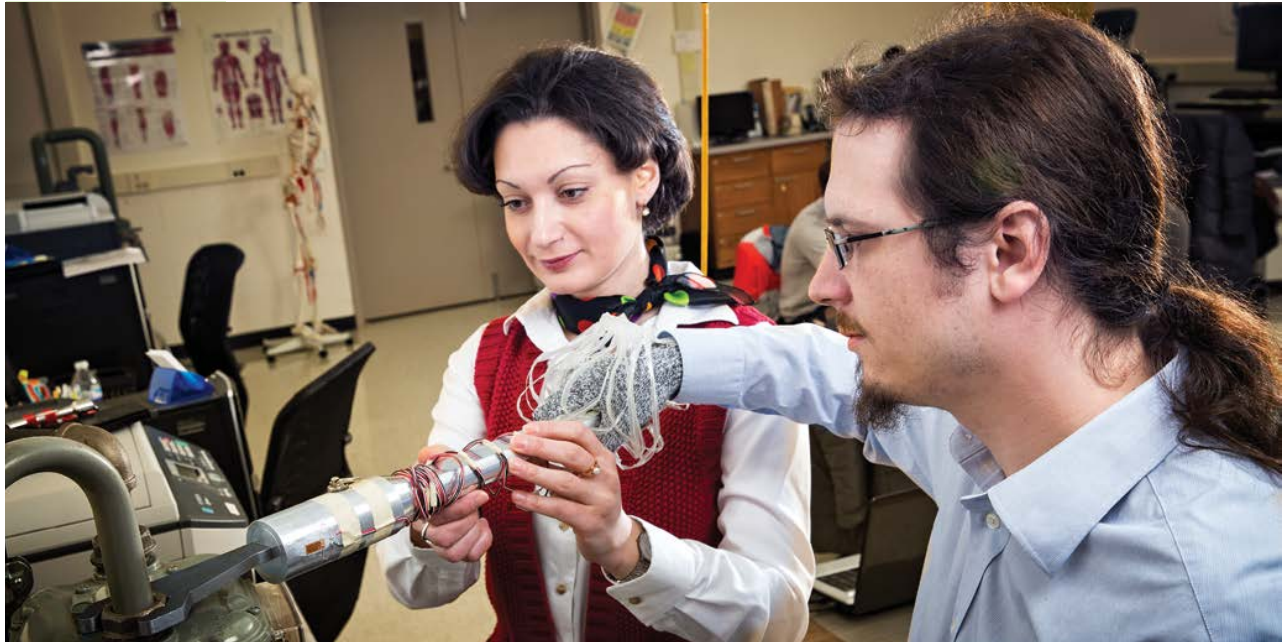
Patrick Dix, a UWM graduate student in industrial engineering, tests a new type of wrench aimed at reducing worker injuries as UWM Professor Naira Campbell-Kyureghyan adjusts a sensor used to measure muscle activity.
