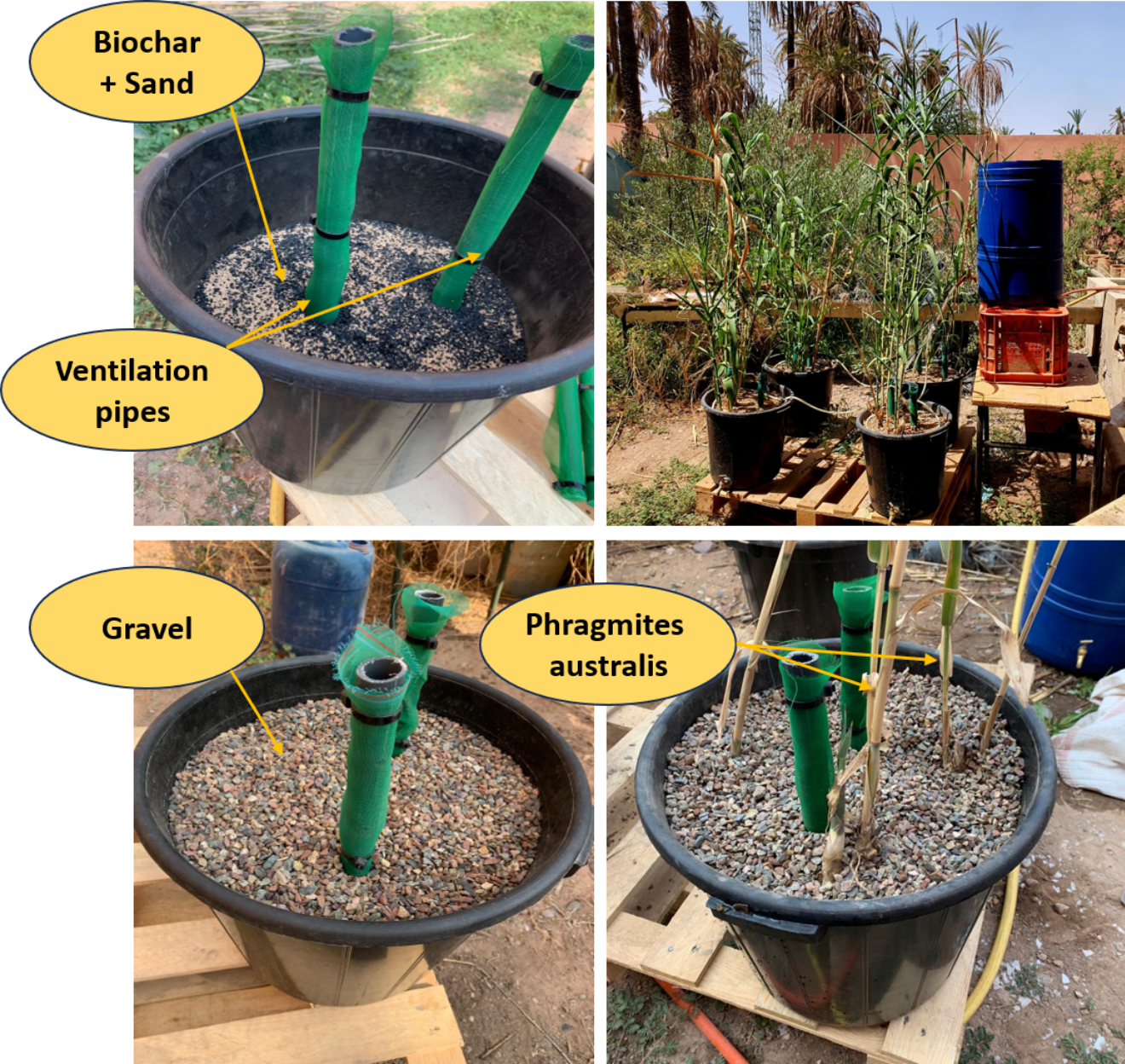
Figure 1 – View of the VF-CW experimental setup.
