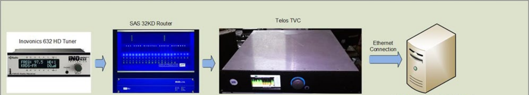
Block diagram of test setup for evaluating audio files that were bit rate reduced AFTER watermark encoding
