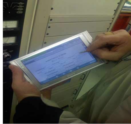
Figure 1. Portable Sony Location Free TV Web Browser being used for data entry into the electronic maintenance log
