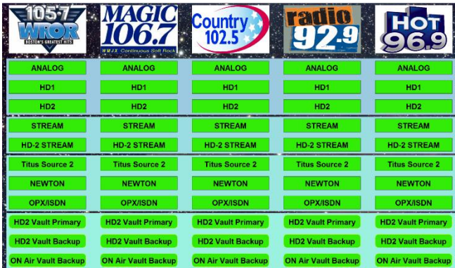
Fig 6 30-inch computer screen showing the confidence of PPM watermarking for multiple audio sources over multiple stations. Green indicates high confidence
