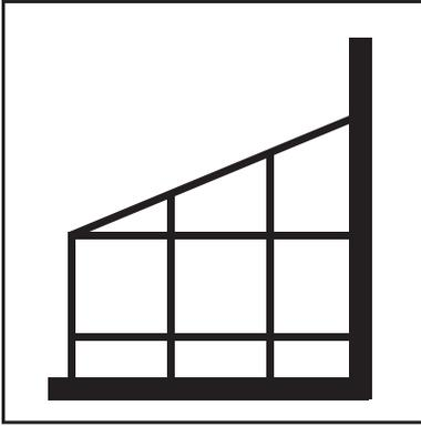
**11. Three Season Room:** Use minimum expansion space of ½". Climate conditions should be between 55° & 80° F and 30 to 55% relative humidity 48 hours prior to, during the duration of the installation and 48 hours after the installation is completed.
