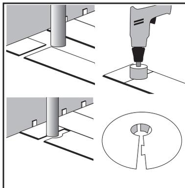
**18. Installing Around Pipes**
