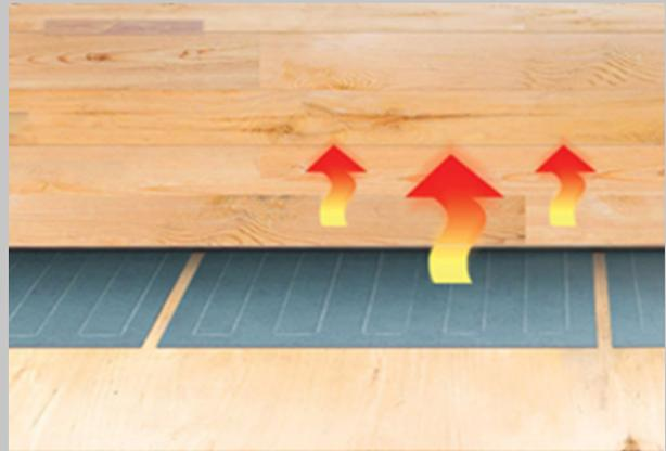
Since the heating mat with thermal cut-off is being installed at the same time as the floor it eliminates pre-running the system. Preheat the room to 10° F below desired room heat. Set floor thermostat to 5° F above its current temperature, and increase 5° F daily, until desired thermal comfort is achieved.
