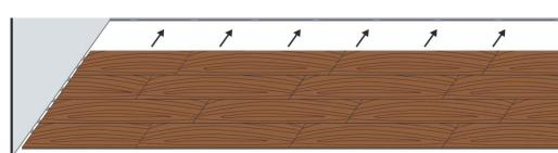
Continue with the installation throughout the rest of the room. When you get to the final row, measure the distance to the far wall and 'rip' a row of boards to fit the gap remember to leave 3/8" (8mm) expansion space against the far wall.
