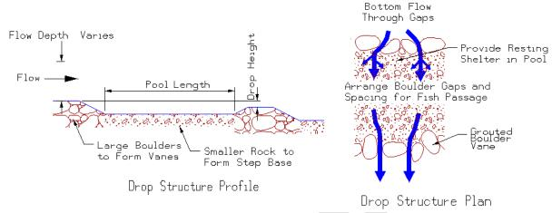
Figure 33. Profile and plan view of a drop structure drop
