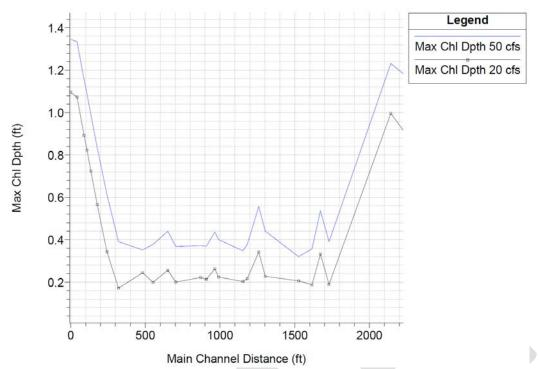
Figure 8. Estimated depth of flow on Little Goose Creek during low flow periods
