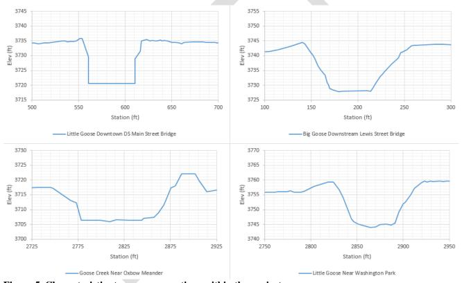
Figure 5. Characteristic stream cross-sections within the project area
