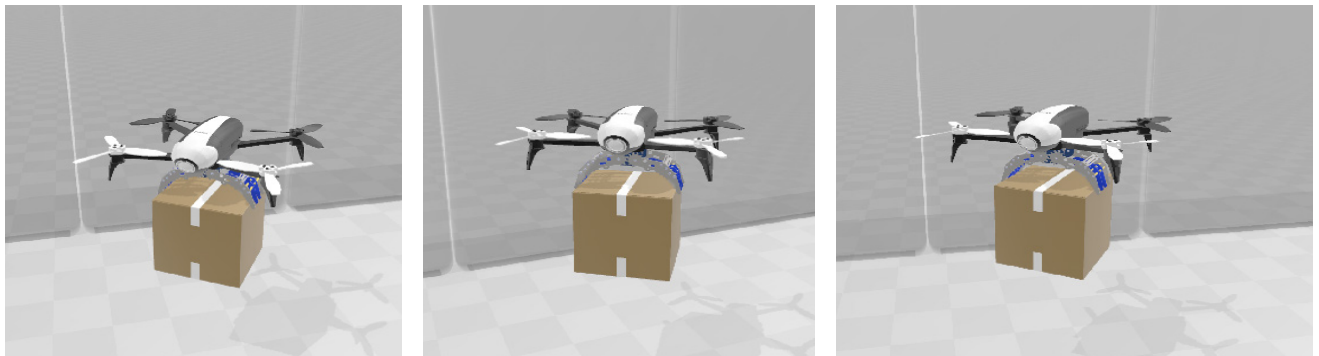
Figure 1 Multi-rotor UAV equipped with a gripper.
