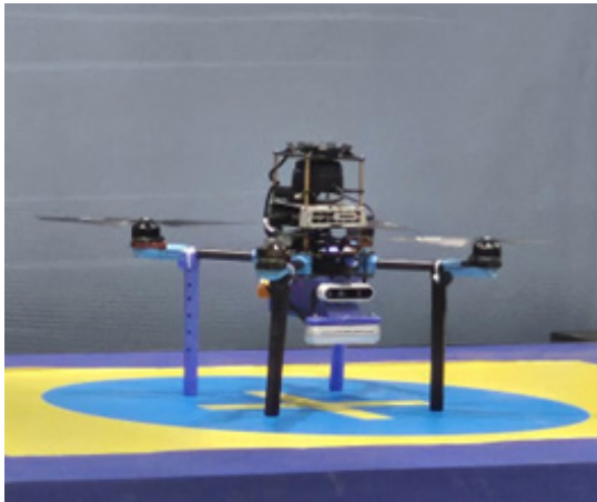
Figure 1 The x500 quadrotor used by the 2023 FRTL winning team Capybots.
