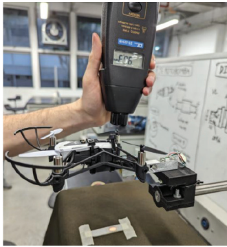
Fig. 2. Indoor experimental setup for real-flight validation of the Parrot Mambo micro-UAV.
