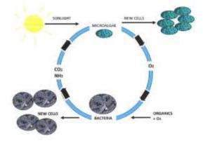
multi-species, single-cell, and oxygen producing algae into the primary cell of a lagoon system. When these microalgae are exposed to sunlight, cultivated and then metered into a
