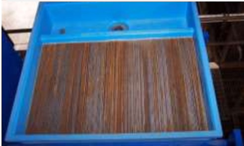
30 gpm EC Chamber with Metal Blades Prior to Wastewater Flow
