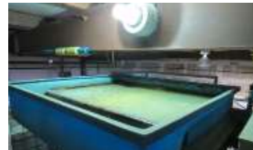
30 gpm EC Chamber with Contaminated Water Flowing through Sacrificial Metal Blades
