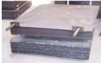
30 gpm Carbon Steel Blade with Cathode and Anode Posts
