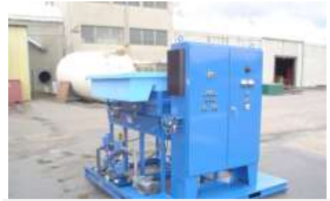
30 gpm EC Power Supply and Chamber
