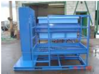
30 gpm EC Chamber, Power Supply, and Observation Deck
