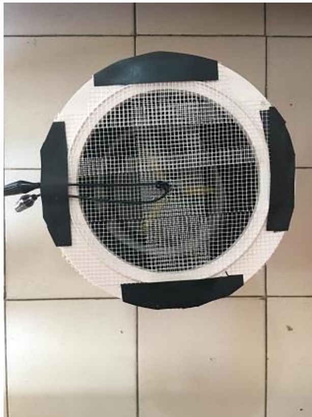
Filter from an Hepa Air Purifier obtained from a junkyard – fitted with extra gauge inside to prevent 'backflow'
