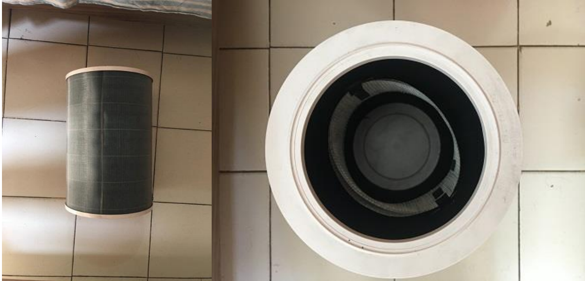
Filter from an Hepa Air Purifier obtained from a junkyard – fitted with extra gauge inside to prevent 'backflow'
