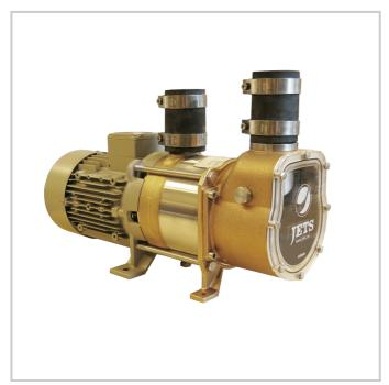
Vacuumarator™ pumps are the most compact, efficient and reliable vacuum generators available for vacuum sanitary systems. The pump creates vacuum, macerates sewage and discharges in one single–pass operation.
