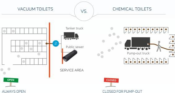
With our flushable vacuum toilets, wastewater flows at great speed to a single, centralized discharge point with every flush. The discharge point can be located far away from the toilets.
