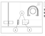
If using Installation Alternative 2, affix the cap (A) from the pipe cover 6 to the wall. (B) will be installed later.
