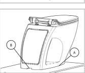
If using Installation Alternative 2, use a cutting knife to cut out the pipe access hole (A) in the back cover A.
