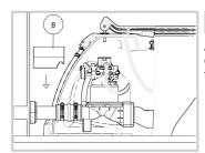
7 Adjust the length and install the pipe cover (B) between the toilet bowl and the wall to cover the connections.
