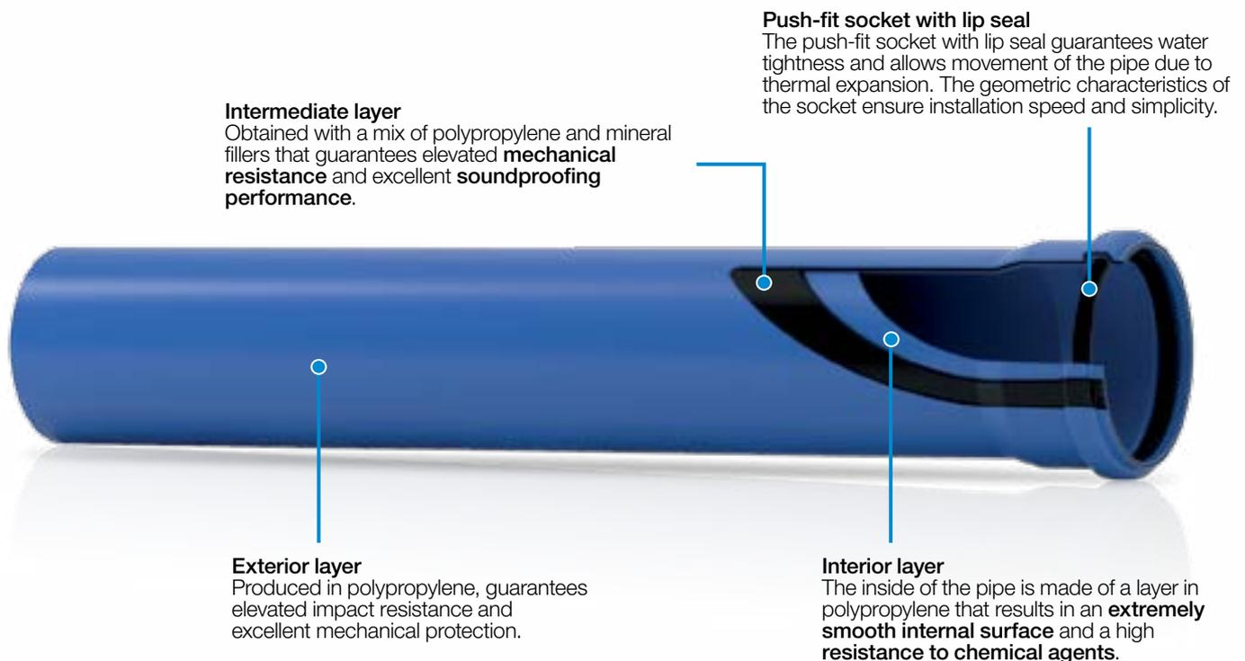
The intermediate layer is created with a **patented polypropylene-based (PP) mix with mineral fillers (MF)** such as to provide the Triplus® system with excellent mechanical characteristics at low (impact resistance at temperatures as low as -25°C) and high temperatures (continuous discharge with temperatures as high as 95°C).
