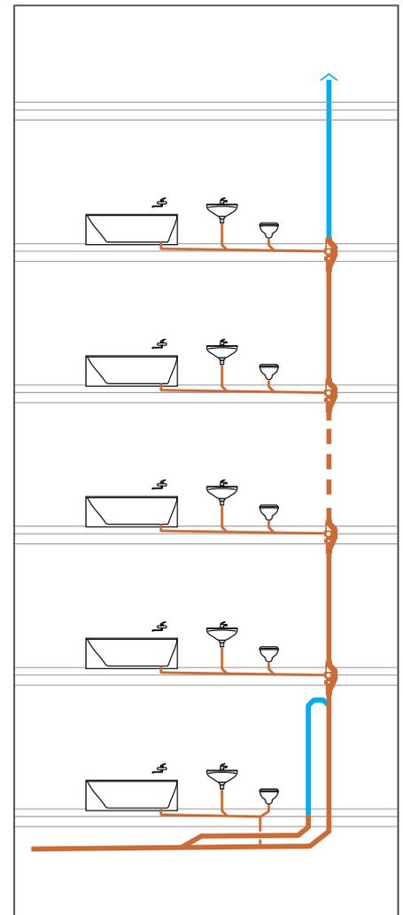
Drainage capacity **40% greater** than systems with primary ventilation.
