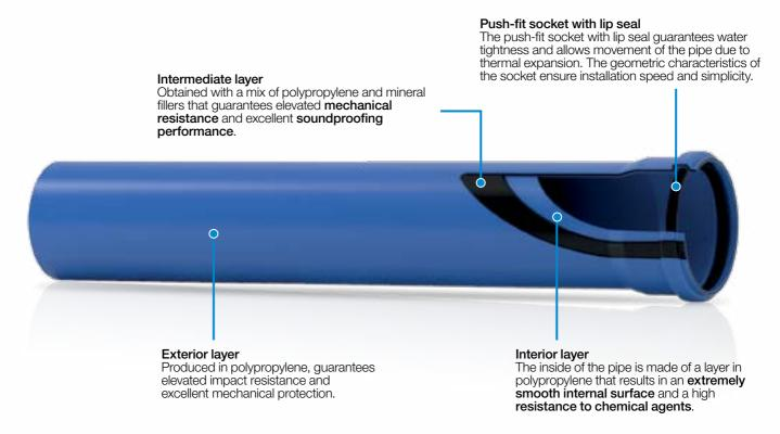
The intermediate layer is created with a **patented polypropylene-based (PP) mix with mineral fillers (MF)** such as to provide the Triplus<sup>®</sup> system with excellent mechanical characteristics at low (impact resistance at temperatures as low as -25°C) and high temperatures (continuous discharge with temperatures as high as 95°C).
