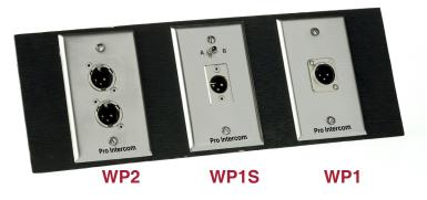
These US-made brushed aluminum plates are fitted with genuine Neutrik<sup>®</sup> XLR connectors firmly machine riveted into place, and are designed to fit standard US single-gang electrical boxes. For greater security, add your own tamper-proof (6-32) mounting screws. Google it; there are many; including Leviton.
