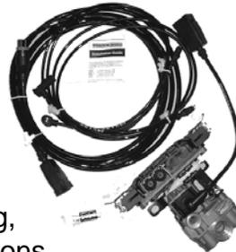
The R955382 kit has no sensors so that the existing sensors can be used if the existing sensor numbers are 10800126 (Wabash number), or S4410328080 (Meritor number.)
