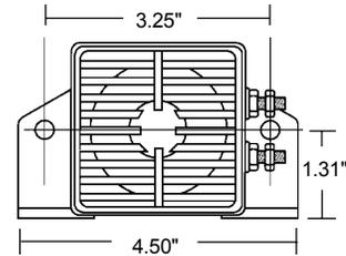
**Part No. FS255** -Fast sounding alarm for special applications requiring a unique sound option. This alarm is capable of quickly demanding attention with sound pulses at 10 bursts per second.
