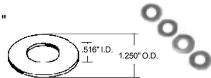
**Nylon Hinge Bearing Washer**
