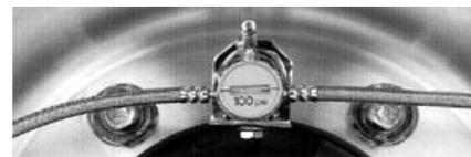
Mounted correctly, Crossfire's yellow indicator verifies that air is flowing freely from one tire to the other, equalizing the load, with just a glance from up to 20 feet away.
