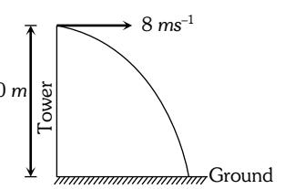
$$\text{Distance, } d = u \times t = 8 \text{ ms}^{-1} \times 4 \text{ s} = 32 \text{ m.}$$
