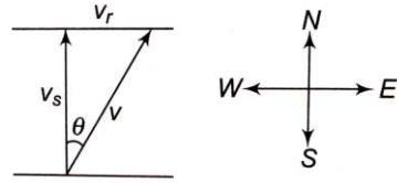
Here, Velocity of water flowing in river,  $v_r = 3 \text{ ms}^{-1}$  Velocity of swimmer in still water,  $v_s = 4 \text{ ms}^{-1}$  From figure, the resultant velocity of the swimmer is
