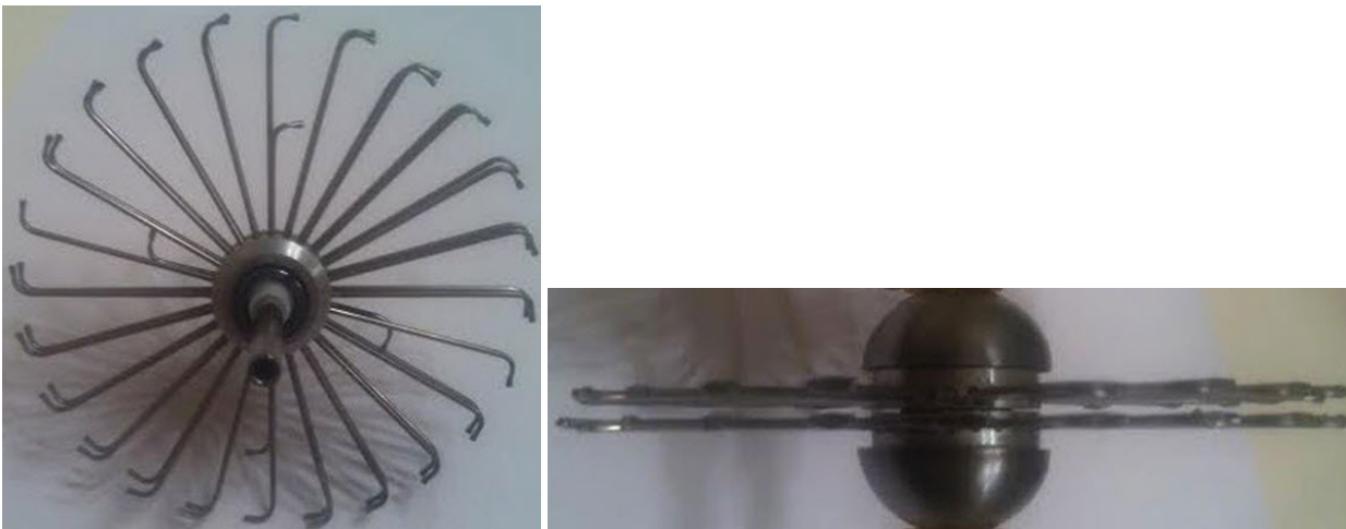
Fig.1 SuperHero Tipjet Reaction Microturbine
