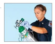
Note: When breaking down the oxygen equipment, be sure to bleed the pressure regulator by turning on the flowmeter after the cylinder has been turned off.
