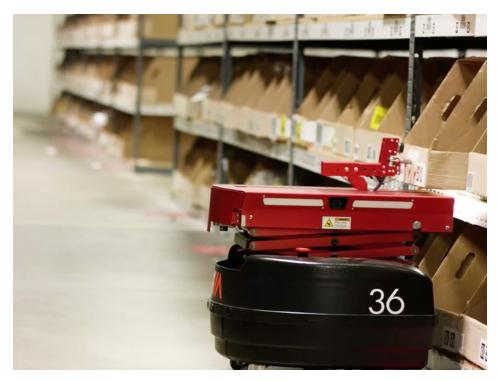
inVia robots are compact but can reach up to eight feet high for picking. | Credit: inVia Robotics
