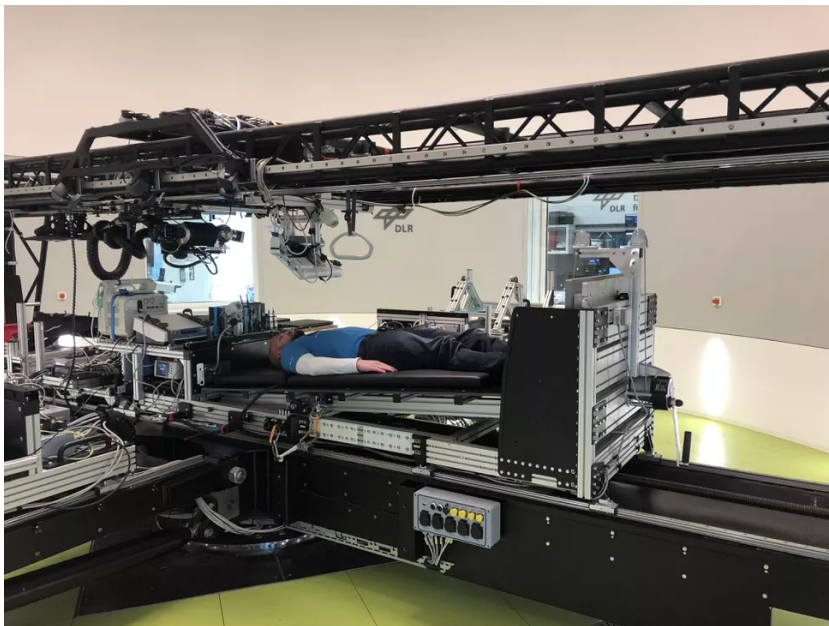
Some study participants will be spun in a short-arm human centrifuge that generates artificial gravity.
