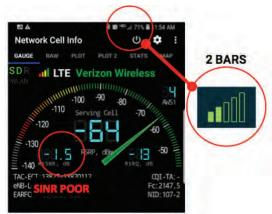
STRONG:: -64 dB Received Signal Strength POOR:: -1.5 dB SiNR Signal Quality
