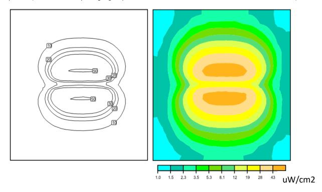
As can be seen, the irradiance values vary quite substantially from the center to the edges. In order to evaluate the setup one has to fix one of the remaining variables: reduction rate (aka log) OR time of exposure. Usually one will start with reduction rate of a specific pathogen. So, if we choose the Escheria coli and want a 99% reduction in the center, we calculate the necessary time:
