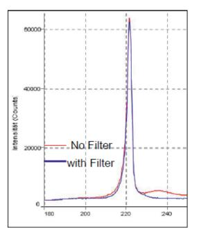
Figure 2: Spectral graph of Excimer lamp with and without short pass filter
