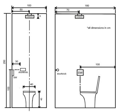
Figure 9: Dimensions of experimental setup in bathroom stall
