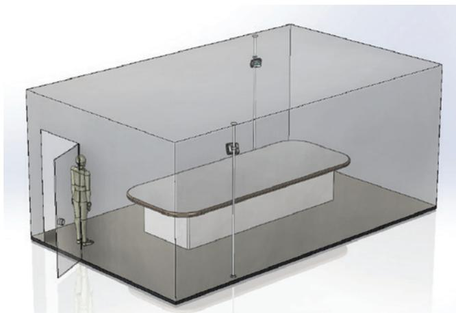
**Figure 5: Position of Care222 module in Room 1**
