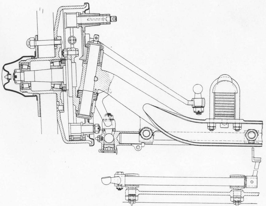
General arrangement of front axle and brake.
