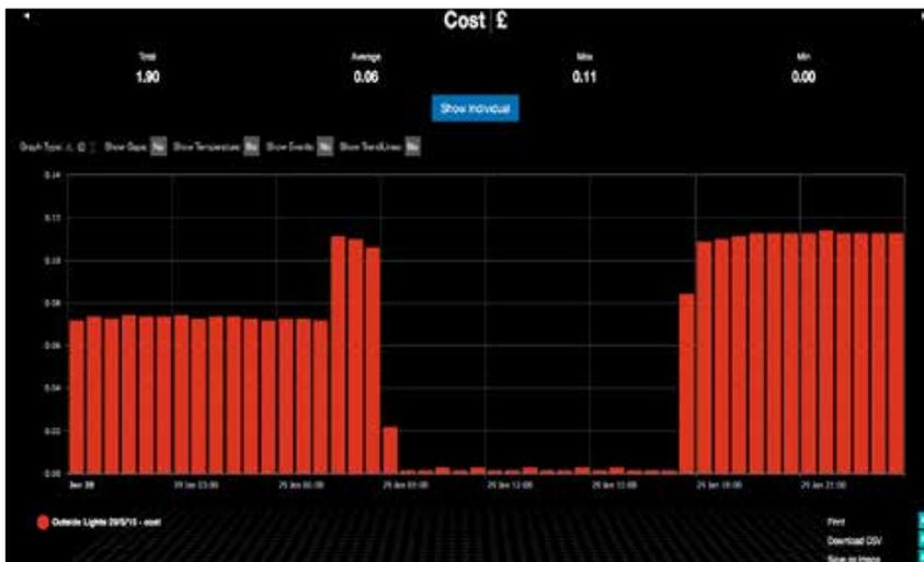
Eniscope Dashboard isolates the running cost of the lighting
