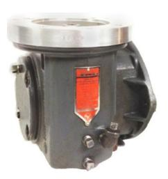
Fill gearbox with recommended, 1 pint, 150W oil before installing onto pinspotter
