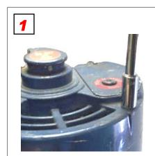
Using a 5/16 nut driver, remove four (4) through bolts and carefully lift Stator from Gear Box Assy. 2
