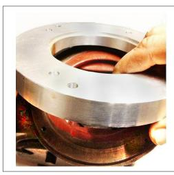
Install the gearbox conversion Adaptor Plate to the register assembly with the four supplied hex head cap screws.
