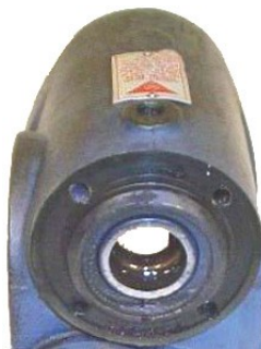
Inboard worm shaft bearing and seal
