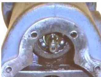
Rear worm shaft bearing
