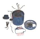
Combo motor *stator* disassembly completed.
