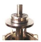
Install stator and new end shield onto rotor shaft and gearbox procedure not shown.
