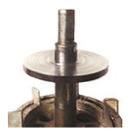
Press *bearing* onto shaft against *brake disc*.
