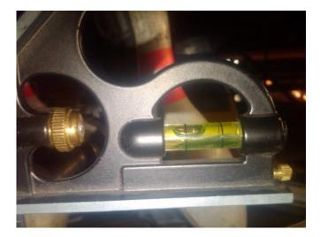
Now you can tighten the Jam nut back up and reposition the collar.
