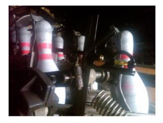
Loosen the Jam Nut and adjust the stop screw until the level on your Tri-Square reads somewhere between center and a 1/2 bubble to the rear of the machine.
