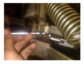
Note: Don't forget to check that the large tension spring on the front leg by the stop screw that you just adjusted is tightened down all the way.
