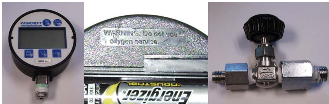
Figure 4. Incompatible oxygen gauge and valve not designed for oxygen service
