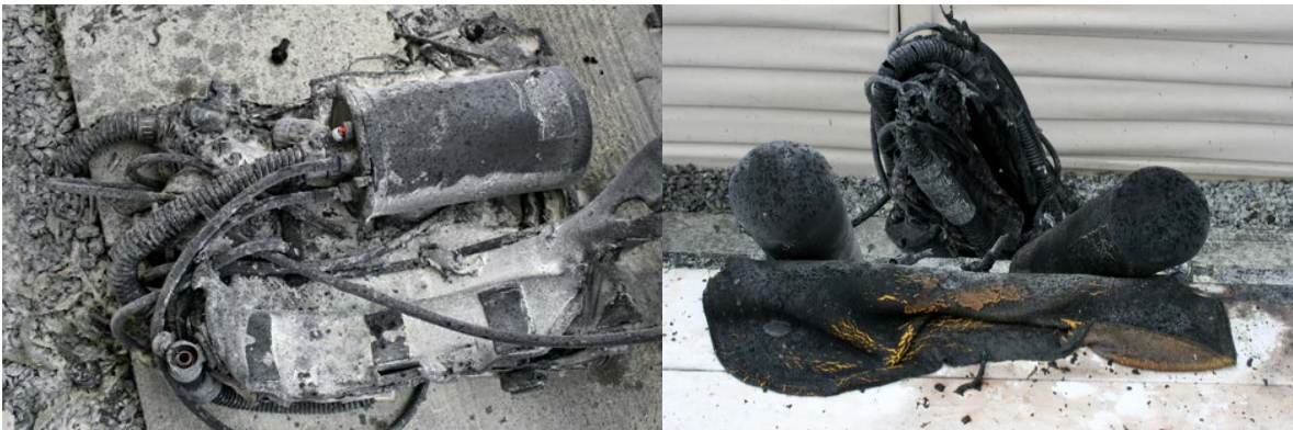
Figure 2. Results of small, localized rebreather fire.
