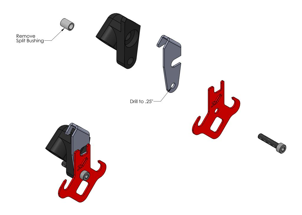
XIHD1-2.0 (GEN II) DYNO-BLADE & INDEXING PLATE INSTALL PROCEDURE
