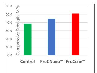
Adding **ProCNano**<sup>™</sup> improved compressive strength by an average of 25.6% vs. control while adding **ProCene**<sup>™</sup> improved it an average
