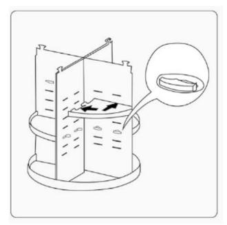
3. Insert the triangle shaped trays into the slots on the plates. Customizable - Arrange them to best fit your planned storage needs.
