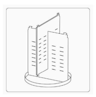
2. Insert the other rectangular plate into the first plate using the center grooves to attach.
