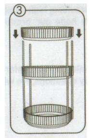
Place the second Circular Upper Plate onto the 4 bars using the holes on bottom.
