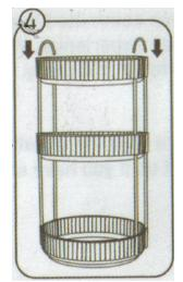
Insert the Small Half Circle Bars into the holes on top of the Circular Upper Plate.
