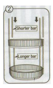
Insert the 4 Shorter Bars into the top holes of the first Circular Upper Plate.
