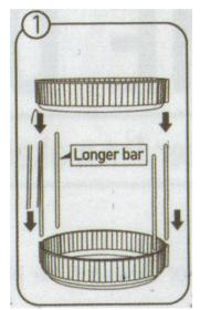
Insert the 4 longer bars into the Circular Rotating Base Plate. Then place the first Circular Upper Plate onto the 4 Bars (fitting the bars into the holes).
