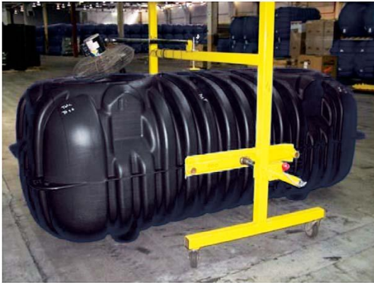
Photo 2.3.4 – Post mold fixturing of Roth tanks
