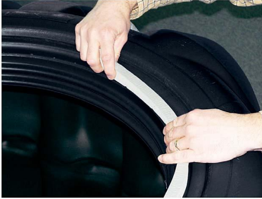
Photo 4.1.17-Applying the foam gasket
