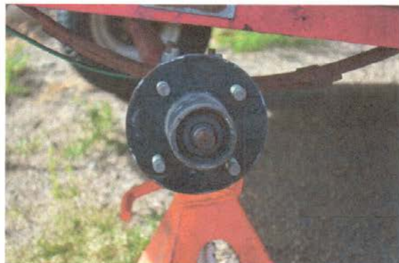
Photo 24 –DSC_0699JPG Right Side Wheel Assembly – Bearing frozen to Axle
