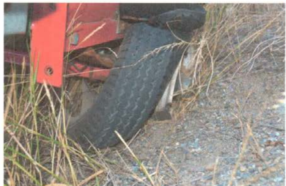
Photo 30—DSC_0118JPG Damage of Right Rear Wheel Assembly discovered approximately 935 feet from Fire Origin
