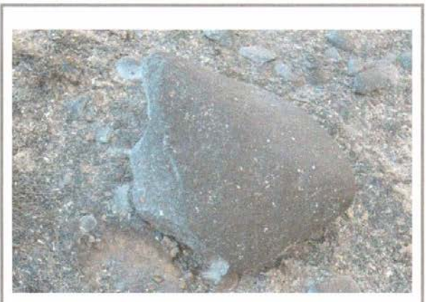
Photo 6 –DSC_0084JPG Advancing Vector – White Ash Deposits located on the origin side of rock
