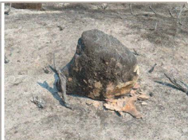
Photo 4 –DSC_200JPG Advancing Vector-Macro Indicator Spalling, Sooting, White Ash Deposits, Degree of Damage
