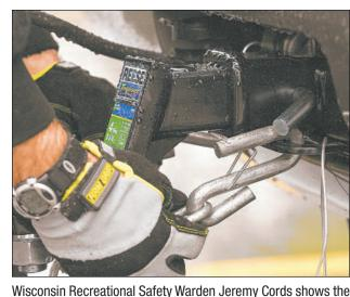
proper method of attaching safety chains when preparing to tow a trailer Friday at the Department of Natural Resources building on Shawano Avenue in Howard. The safety chains are crossed and hooked onto the hitch eyes with a clip that prevents the S-hook from coming free. Jim Matthews/Pressregulations after he hit a up in 2003.
