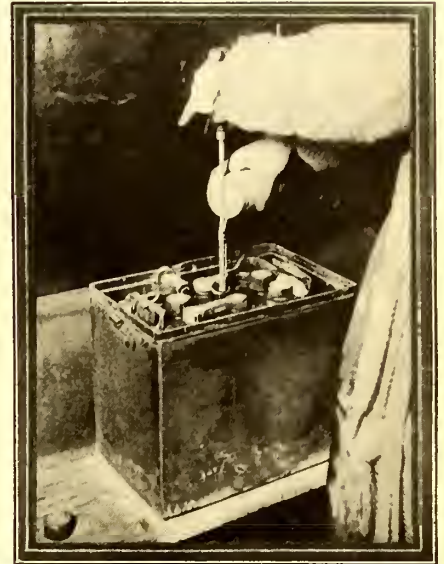
Filling the Battery According to Hoyle Does Not Need an Expensive Equipment. Water May Be Put Into the Battery Safely Without Spilling Over the Cells by Pouring Water From a Glass or Cup Down a Screw Driver, Whose Tip Is Placed in the Cell to Be Filled.
