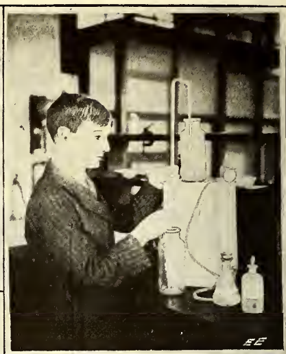
Siphoning Carbon Dioxide Gas. The Candle Test Proves the Experiment.
