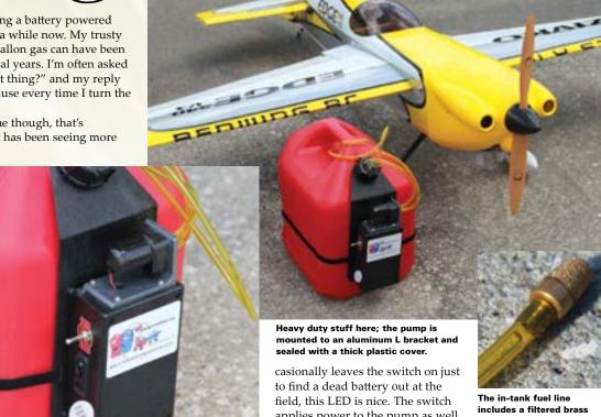
The receiver switch is the master power switch as well as the NiCad charge jack. The heavy duty toggle runs the
