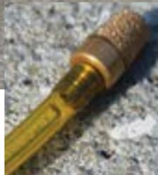
The in-tank fuel line includes a filtered brass clunk.
