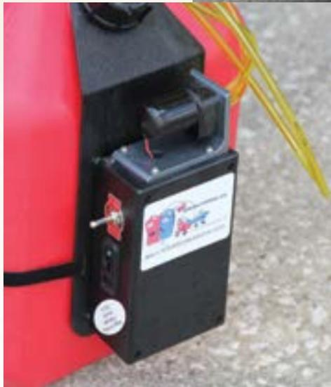
The receiver switch is the master power switch as well as the NiCad charge jack. The heavy duty toggle runs the pump to fill or drain your fuel tank.
